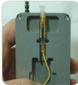
5. Inserting cable(fiber) until bending occurs(important)
