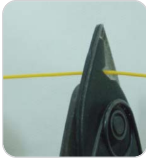
2. Stripping coating around 20mm
