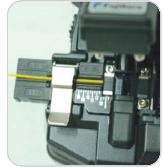
3. Inserting cord after cleaning alcohol and fiber cutting(10mm) using tool
